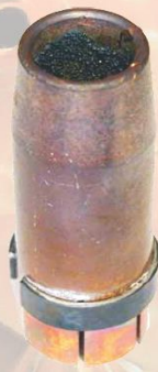
WSS Used, Condition After 4 Shifts
